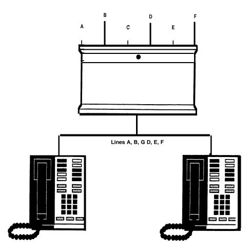
Lines are assigned to the same buttons at each voice terminal. EXAMPLE OF STANDARD SQUARE CONFIGURATION
